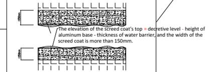
3. Make level with high strength of cement mortar. The width is more than 150mm.
